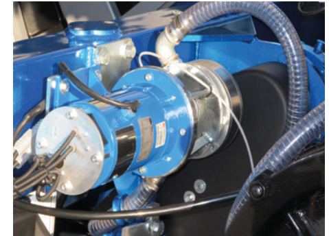
AUTOMATIC SUCTION FILLING Electric motor-controlled vacuum pump to easily and quickly fill the suction hose.
