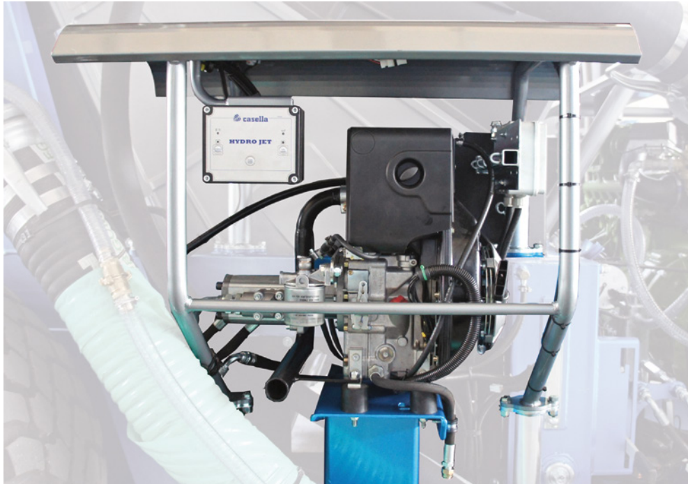
Engine single cylinder for rewinding independent of the pipe
